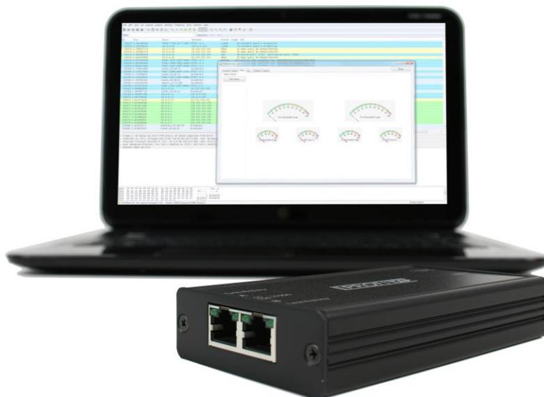
ProfiShark 1G is highly portable and powered through USB 3.0.
